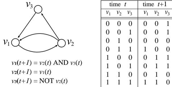
Figure 1. Example of a Boolean network. Dynamics of a Boolean network (left figure) is well-described by a state transition table (right figure). For example, if the state of the network is  $[0, 1, 1]$  at time  $t$ , the state will be  $[1, 0, 0]$  at time  $t + 1$ .
