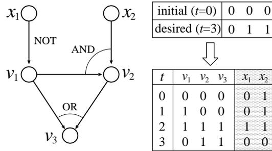
Figure 2. Example of the control problem (BN-CONTROL). In this problem, given initial and final states of internal nodes ( $v_1, v_2, v_3$ ), it is required to compute a sequence of states of external nodes ( $x_1, x_2$ ) that leads to the final state.
