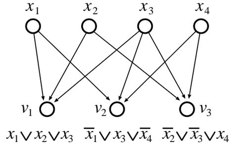
Figure 3. Reduction from 3SAT to BN-CONTROL. An instance of 3SAT  $\{y_1 \vee y_2 \vee y_3, \bar{y}_1 \vee y_3 \vee \bar{y}_4, \bar{y}_2 \vee \bar{y}_3 \vee y_4\}$  is transformed into an instance of BN-CONTROL in a simple way that external nodes correspond to variables in 3SAT and internal nodes correspond to clauses.
