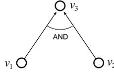
Figure 5. Computation of  $S[v_3, t, 1]$ . In this case,  $S[v_3, t + 1, 1] = 1$  if and only if  $S[v_1, t, 1] = 1$  and  $S[v_2, t, 1] = 1$ .  $S[v_3, t + 1, 0] = 1$  if and only if  $S[v_1, t, 0] = 1$  or  $S[v_2, t, 0] = 1$ .
